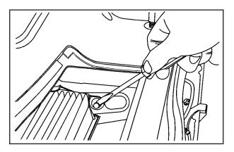
2. Then, insert a tool behind the push pin located on the inboard side of the air filter compartment to carefully pry the pin out.
